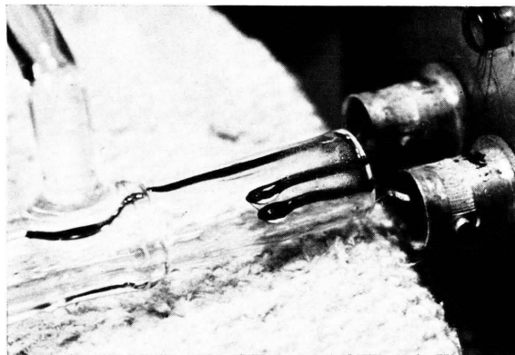
Fig. 1. The electroantennographic detector consisting of an insect antenna placed between two drops of saline solution at the tips of chloridized silver electrodes. Diameter of silver wires is 1.2 mm, antenna shown is of a Lobesia botrana male.
